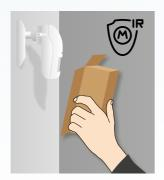
OPAL Pro is provided with an active IR anti-masking function, so it will detect any attempt to cover the detector lens with paint or lacquer, or with materials of different thickness, color and texture.
