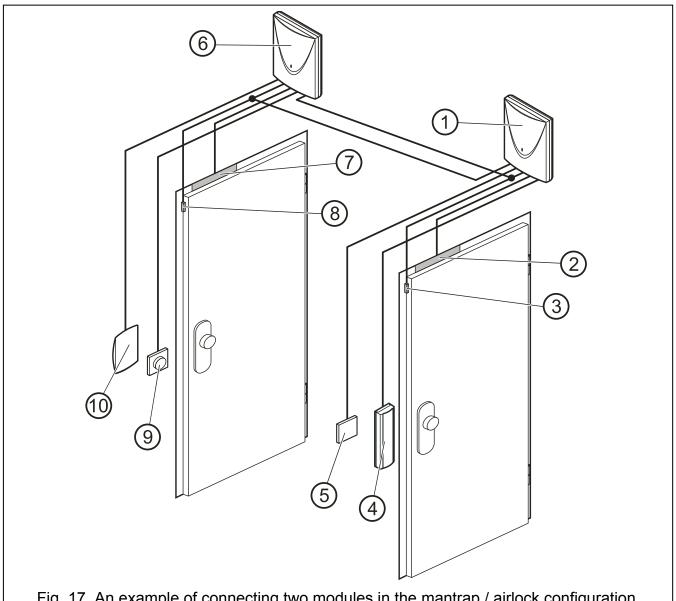
Fig. 17. An example of connecting two modules in the mantrap / airlock configuration.
