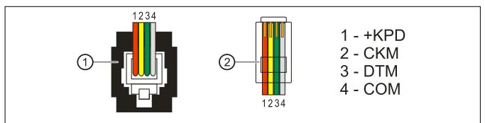
Fig. 15. Sequence of wires in the plug connecting LCD keypad with module. 1 – view of plug in socket. 2 – view of plug from pins side.
