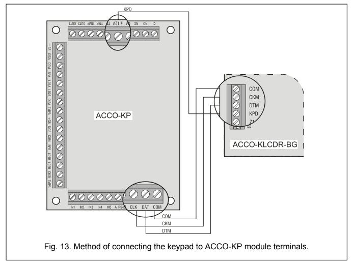
The module supports keypads with addresses 0 and 1. The keypad with address 0 will serve as terminal A (entry terminal). The keypad with address 1 will serve as terminal B (exit terminal). The information whether the keypad performs the function of terminal A
